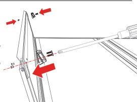
Set the cover (C) in the folded position on the side rails (A & B) towards the cab of the truck. Confirm the cover is evenly spaced between the rails.
