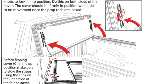
**CLOSING COVER:** To drive with the cover (C) closed, unhook the buckles and straps from the bulkhead. Stow the straps using the clips on the underside of the folded cover. Fold all panels towards the tailgate making sure that all latches are engaged.
