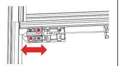
With the latch cover removed, loosen the screws and move the latch bracket to adjust. Retighten the screws. Slide the latch housing back on.
