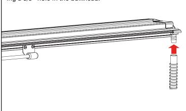
Place the passenger side rail (A) on the truck rail.
